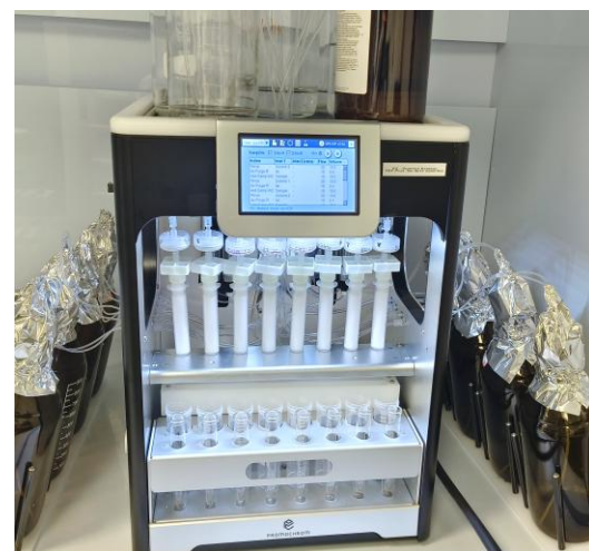
SPE-03 with Mini-disks and inline drying columns
